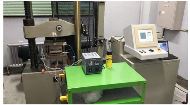
Fig. 5 Photograph showing deep drawing die and universal testing machine.
